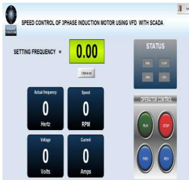
**Fig. 3** SCADA screen shot of animation of real-time control setup
